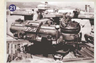
This large German anti-aircraft rangefinder was mounted on the roof of the tower now known as the 'Odeon'.
